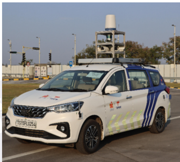
Figure 3. SAFARI – TiHAN IITH Data Collection Vehicle
